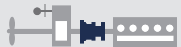
Auxiliary drive via PTH/PTI in case of main engine failure. The vessel remains maneuverable.
