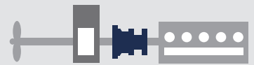
When the KAZ is disengaged, the shaft generator can be used as PTH/PTI for back-up propulsion of the vessel.
