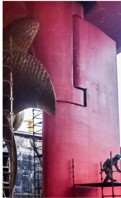
*“Highly qualified professionals with FROSIO red level certificates evaluated the coating and gave the green light for application. After five years of operation at various speeds there were only minor detachments and those were easily repaired.”*
