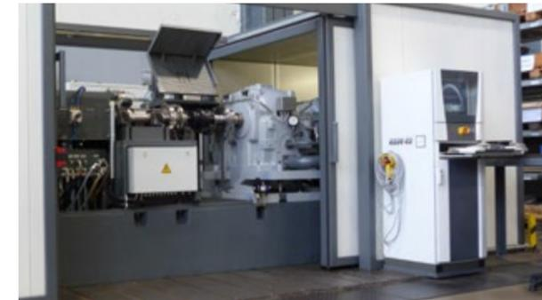
To verify the calculations and design of the couplings before commencing with serial production, RENK AG Rheine Works uses several test benches with which it is possible to simulate almost all static and dynamic loads as well as drive profiles during railway applications. With fatigue analysis, the specified lifetime can be reviewed in a test phase.
