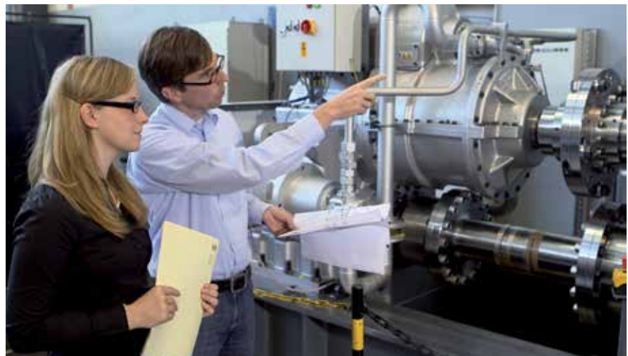
Back-to-back testing of a T 2 RECS 560 LL
