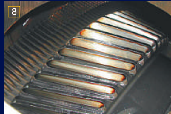
Picture 8: Bad lube oil maintenance however 23 years of troublefree operation in water power.
