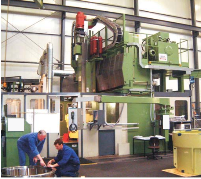
1 CNC gantry drilling machine
