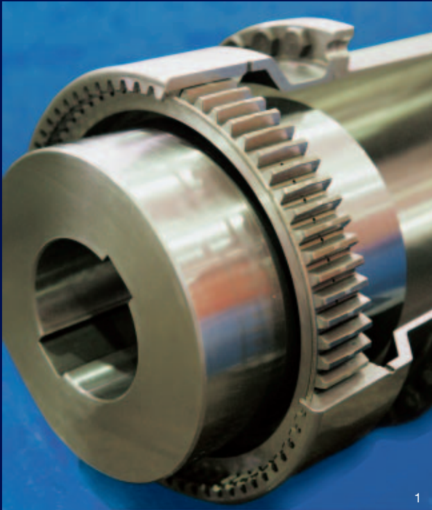
1 Curved Tooth Coupling with hardened and ground inner and outer teeth, tooth-by-tooth injection lubrication
