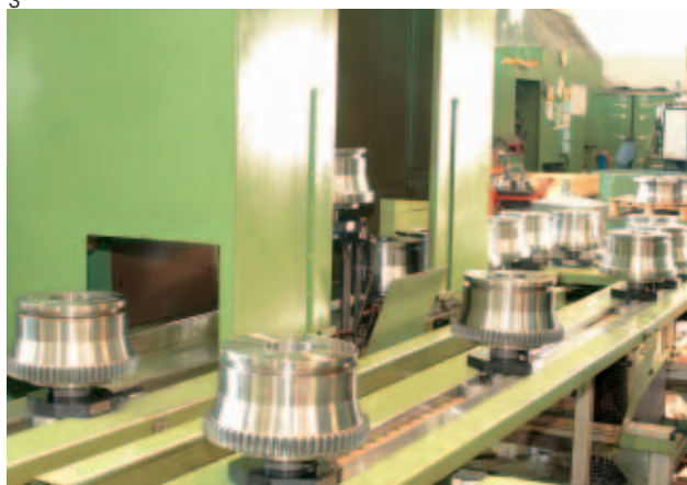
1 Gear slotting machine for the production of internal curved teeth
